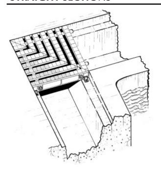
The modular, interlocking grate corners are preassembled in one foot sections. Always commence at one point (corner) and add only in the same direction to come back to the starting point.
