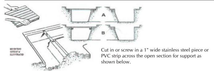
Lay in the first piece of grating, anchor down and continue laying in the same direction. To end up at the exact length, cut or grind the male ends of the last few bars to narrow up the spacing.
