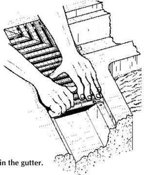
Lay the first section in the gutter.
