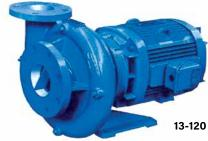
**PACO MAIN CIRCULATION PUMPS** End suction centrifugal pumps custom designed to meet your pool's exact flow and head characteristics. Available in cast iron or all bronze and single phase or three phase. Capacities up to 4100 GPM, heads to 800! Sizes 1" to 10" (discharge) and  $V_3$  to 125 HP. **NSF approved models available.**
