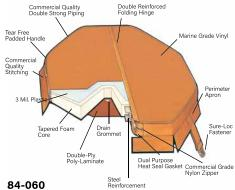
**INSULATED SPA COVER** – 4" to 2" tapered foam core for excellent insulation. Covered by a marine grade vinyl with mildew and UV inhibitors. Double reinforced center folding hinge for easy removal and storage. Steel reinforcement rib for strength and rigidity. Cover mounts on lip of spa or on coping. Floating cover can also be used on water surface to increase insulating capabilities. Available in 10 different colors.
