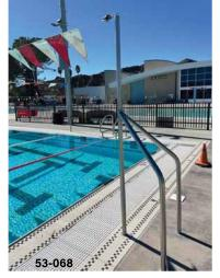
FALSE START STANCHIONS - 4'6" high round stainless steel tube capped at one end with a stainless steel closure plate and U-hook for recalling swimmers. Placed 36' from end of the pool. Two posts required. Stanchion only. Sliding collar with eyebolt and post anchor ordered separately.
