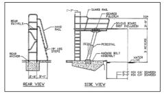
**THREE METER DIVING STANDS** – Stands come in three grades, Ultraflyte, Superflyte, and Topflyte. Diving board ordered separately. Specify brand and length of diving board to be used and pool deck-to-water level dimension when ordering.
