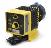
LMI B SERIES & C SERIES CHEMICAL FEED PUMPS — Electronic solenoid driven chemical feed pumps with variable speed and stroke length adjustments. Rugged chemical resistant housing for corrosive environments and chemicals. Four Function Valve AutoPrime liquid end allows for de-gassing during pump priming and operation when used with Sodium Hypochlorite (Bleach).
