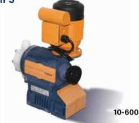
**PROMINENT SIGMA FEED PUMPS** Mechanically-actuated diaphragm pumps. Pumps are programmable and display comprehensive data for monitoring and recording. Functions include: digital setting of stroke frequency, manual stroke length adjustment, integral variable speed and access codes. Designed to be hard plumbed. 3/4" MPT connections, 115 volt, 60 Hz. NSF 61 Listed.
