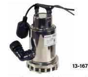
PENTAIR STAINLESS SUBMERSIBLE PUMP — Utility drainer pumps water down to 13/8" in depth. Stainless steel casing, suction strainer, clog-resistant impeller and shaft, for corrosion resistance. External float switch included. 15 ft. power cord. 115 volt/60 Hz. 13-167 1/2 HP
