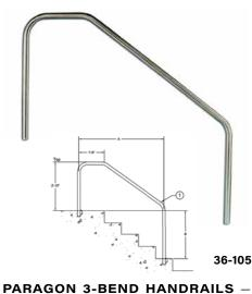
3-Bend Handrails feature a 18" horizontal transition to the sloping portion of the handrail. Handrail allows you to have safe access to your pool. Front leg requires underwater anchor socket. Stainless steel 1.90" O.D. tubing x .065", .109" and .145" wall thickness. Requires two anchors and escutcheons (extra).
