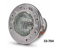
**PENTAIR AQUALIGHT** — The AquaLight uses halogen quartz bulbs and is designed for installation in small plastic or stainless-steel Pentair niches. The light shell is high-quality stainless steel, and the lens is prismatic tempered glass. Easy service stainless-steel clamp. Low water cutoff. Easy to service. Plastic snap-on face rings and colored lenses available. UL Listed.
