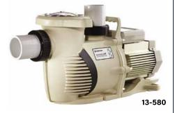
PENTAIR WHISPERFLO XF PUMPS Whisper quiet, self priming pumps with high efficiency performance are ideal for commercial applications. Large capacity hair and lint strainer with see through lid. 2.5"/3" union connections. Available in 208-230 volt/single phase or 208-230/460 volt/three phase with TEFC motors. NSF Listed.
