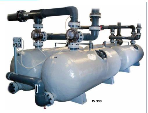
**STARK A, B, AND C STYLE SYSTEMS** — Includes side mounted manhole with viewport, Schedule 80 PVC face piping with flanged connections, water actuated backwash valves, manual multiport valve, influent/effluent pressure gauges, automatic air relief and backwash sight glass. UL Listed Automatic Backwash Controller (24VAC) is available as an option.
