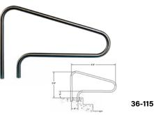
**PARAGON DECK-MOUNTED HORIZONTAL RAILS** — Deck Mounted Rails allow you to have safe access to your pool without the need for an underwater anchor socket. Stainless steel 1.90" O.D. x .065" wall thickness. Requires two anchors and escutcheons (extra).
