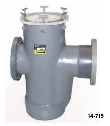
LARGE PORT FIBERGLASS STRAINERS Composite strainer body with fiberglass reinforced plastic (FRP) and PVC material. Same features as our Fiberglass Basket Strainers, but includes large outlet design. Includes clear acrylic cover with easy open tee handles. Available in straight in-line style and eccentric reducing style. Inquire for additional sizes and styles not listed. Rated to 50 psi.
