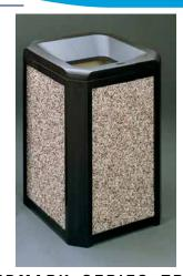
LANDMARK SERIES TRASH **CONTAINER** – Large opening funnels refuse into container and out of view. Hood is hinged and includes a stay open trap for easy access to rigid liner. Container color: Sable. Size: 26" square x 301/2" H (35 gal.) Includes Rigid Liner. Aggregate panels ordered separately. Panel Colors: Brownstone, Riverrock, and Coral.
