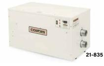
**COMMERCIAL ELECTRIC POOL/SPA HEATERS** Medium duty pool and spa heaters with built-in flow switch. Operating range: 20-80 GPM. Includes: Incoly heating elements, stainless tank, digital thermostat, manual reset hi-limit switch, flow switch, and element, flow and high temp "on" lights. 24/30 KW units (CPH Series) with 1<sup>1</sup>/<sub>2</sub>" male NPT connections. 36 KW and higher units (PHS Series) have 2" male NPT connections. UL Listed for indoor/outdoor installation.
