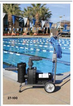
**LINCOLN PORTABLE PUMP SYSTEM** — Allows you to vacuum and discharge debris to waste. System features stainless steel cart and rubber wheels, pump with clear-lid strainer basket and vacuum priming "T." Includes: (2) 1½" and (2) 2" hose connection fittings. Electrical pumps include in-line GFCI and watertight power switch. Pump Overhaul Kit includes: impeller, shaft seal and "o" ring.
