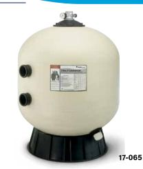
**PENTAIR TRITON FILTERS** – Patented one-piece fiberglass tank with UV protected surface. Top loading with swing-away diffuser for instant access to sand bed. Available with 2" threaded or 3" flanged tank ports. TR 140C / TR 100C commercial models have larger 8" opening, 3" flanged connections, and 2" drain. Tandem plumbing kits and automatic backwash controls available. Backwash valve and media extra. NSF Listed.
