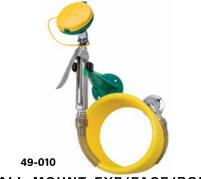
WALL MOUNT EYE/FACE/BODY SPRAY HEAD — Allows user the ability to wash all parts of the face and body. Easy-to-use spray unit features a chrome plated squeeze lever for one-handed operation. Single spray head has automatic pop-off dust cover. Vacuum breaker is required on all hand held eye/face/body spray units per local code, not included. Includes: wall bracket, 12' recoil hose and universal sign. 49-010
