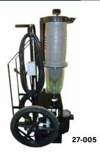
**CYLCLONE PORTABLE VACUUM** — 1 HP portable vacuum system with 50 ft. cord. Mounted on a powder coated portable cart, with non-me-tallic, chemical resistant wheels. 75 sq. ft. cartridge filter with Multi-Cyclone debris separator, which extends the time between filter cleanings 4-6 times. 110 volt with 20 amp GFCI.
