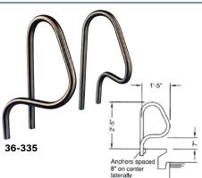
**PRETZEL BEND GRAB RAILS** – Requires the least amount of deck width with the narrowest profile as the legs are offset laterally instead of front to back. Requires four anchor sockets, four escutcheons, and recessed steps as needed (extra).
