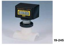
**BLUE-WHITE F1000 DIGITAL FLOW METER** — Battery operated digital flow meter and flow totalizer. Tamper-proof, ABS, NEMA 4X enclosure. Clear 6 digit LCD display. +/- 2% accuracy. PVDF saddle mount (2"/ 3") or Sch. 80 PVC saddle mount (4"/ 6" / 8"). Operates on 2 AAA batteries, included. Also available, as flow rate only or flow totalizer only meters, inquire.
