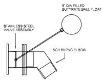
**YMCA STYLE FLOAT VALVES** — Modulating float valve for use in surge tanks and open top Vacuum D.E. filters. YMCA style encases float valve in PVC pipe, with angled diversion plumbing and flanged connection. Float arm, shaft, and disc are stainless steel, with black plastic float ball.
