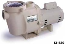
PENTAIR WHISPERFLO PUMPS -High efficiency, self priming, single speed pool pumps, with large strainer basket and see-thru lid. High efficiency impeller create maximum water flow, while minimizing turbulence and noise. Energy efficient, single speed motors, with commercial grade frame. 2" suction/discharge ports. Available with TEFC three phase motors. NSF Listed
