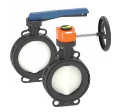
**PLASTIC BUTTERFLY VALVES** — High performance thermoplastic butterfly valves and stronger and 60% lighter than metal valves. High quality, Swiss made, Butterfly Valve Type 565 is the same installation length as metal valves, for easy replacement. Materials of construction-PVDF disc, with EDPM sleeve, and fiber reinforced housing and inner disc. Available in manual lockable hand lever or gear operated with hand wheel style valves. Mounts between two pipe flanges, ordered separately.
