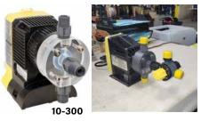
**LMI PRIMING VALVES** – These multifunction valves come with a ½" discharge connection. They can be adapted by using the appropriate tubing connection kit. Ordered separately.
