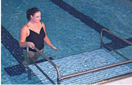
ADJUSTABLE HEIGHT TEACHING PLATFORM — Provides a secure, elevated surface for your lesson programs. Stainless steel with non-skid cross-grooved sand textured deck. Legs are adjustable in 2" increments via quick release pin with five height positions. Platform places swimmers 18" - 26" above pool floor. Size: 60" x 30". Includes easy grip rails on 3 sides for added security. Weighs 175 lbs. **56-060** Adjustable Height Teaching Platform
