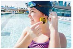
**FINIS TEMPO TRAINER PRO** — The small, waterproof device easily secures beneath a swim cap and transmits an audible tempo beep. Adjustable tempo offers the ability to identify and maintain an ideal pace. Three different training modes offer ultimate customization. Includes a clip for dryland exercise.
