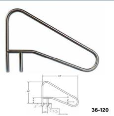
PARAGON DECK-MOUNTED WELDED RAILS — Sloping handrail for pool entry steps provided safe entry and exit from the pool. Welded rail offers greater rigidity than standard handrails. Does not require underwater anchor socket. Stainless steel 1.90" O.D. x .065" wall thickness. Requires two anchors and escutcheons (extra). **36-120**
