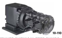
STENNER CHEMICAL FEED PUMPS – QuickPro Series dual head, peristaltic metering pumps. Same as single head pump features described above. 120v/60 Hz. 220v models also available. Includes: pump, spare pump tube, connecting nuts, ferrules, 20' x 3/8" suction/ discharge tubing, injection fitting, weighted suction line strainer, latches, and mounting bracket. Rain Roof for outdoor installation ordered separately. ANSI/NSF STD 50.
