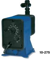
**PULSATRON A PLUS FEED PUMPS** — Electronic solenoid pump with stroke length and speed control. 100:1 turndown ratio. PVC Head. Includes: injection fitting, 16' of tubing, and choice of standard bleed value, 5 function valve with anti-siphon, or 5 function valve with Degas (for sodium hypochloriite) and anti-siphon. Specify chemical being used. 120 volt. **ETL Listed.**
