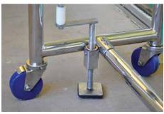
JUNIOR STAINLESS STORAGE REELS For smaller sized pool cover applications. Frame constructed with 1.75" OD x 120" wall thickness 304 stainless steel tubing. Winding tube is made with 4" OD x 120" wall thickness tubing. Includes: 12" hand crank, 2 screw jack brakes, and four 4" diameter stainless casters. Dimensions: 18"H x 24"D x winder length (L). Can hold up to 80 In. ft. of insulating pool cover material. **10 Year** Warranty
